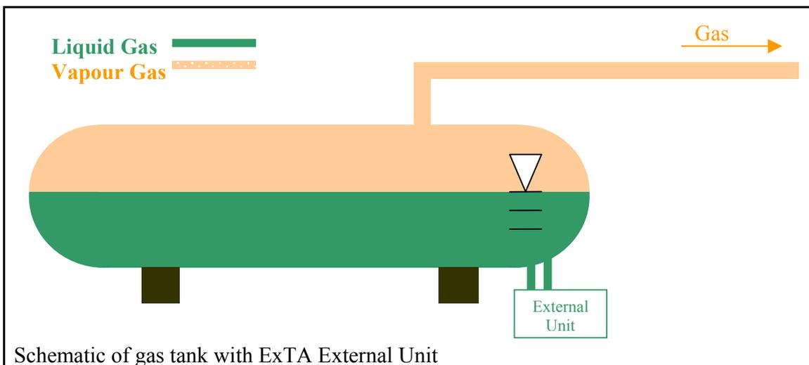
Schematic of gas tank with ExTA External Unit
